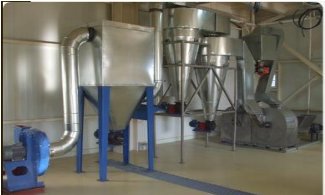
Figure. 3a. General appearance and advantages of Pneumatic (Flash) dryer.
